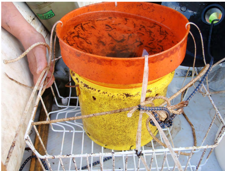
Photo 2: Sediment trap retrieved from Nordic Lake, October, 2012.
