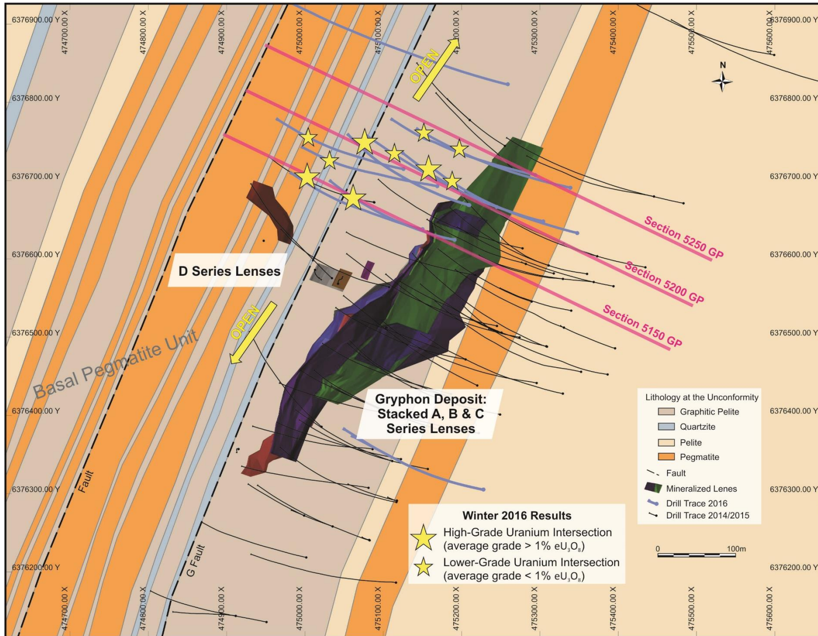
Figure 2: Plan map of the northeast plunging Gryphon mineralized lenses projected up to the simplified basement geology at the sub-Athabasca unconformity
